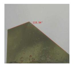
Control and consistency is something electromechanical engraving provides with digital accuracy, but what if your stylus angle changes? Increase the repeatability and consistency of your engraving by tracking your stylus. The Vertex Stylus Monitoring system provides a simple and fast way to monitor the stylus angle, and bring a new level of uniformity to your engraved cylinders.
