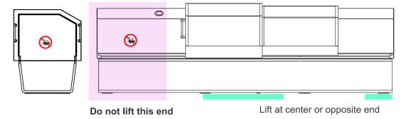
After the machine has been uncrated, move the machine on its skid close to its final location.
